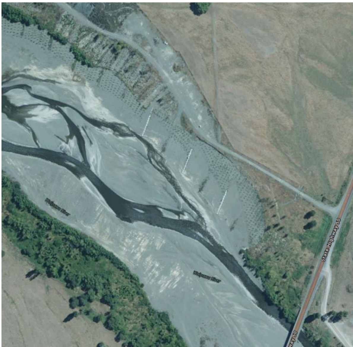
Figure 15. Newly completed Waipawa River training works upstream of SH50 – prior to Cyclone Gabrielle.
