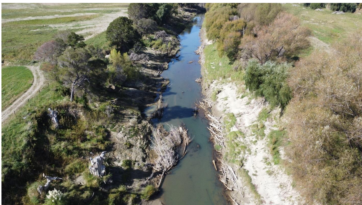
Figure 26. Bank stabilisation by tree willows (right bank) contrasted with slumping into the channel on left bank (despite the presence of mature mānuka and other tree species).
