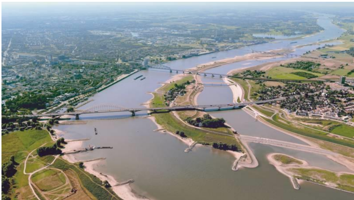
Figure 1-2 River Waal in the Netherlands with newly constructed overflow channel on the right as part of “Making Room for the River” programme
